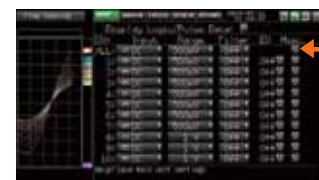
Parameters in AMP settings for 10 channels can be set at once using the ALL field.
